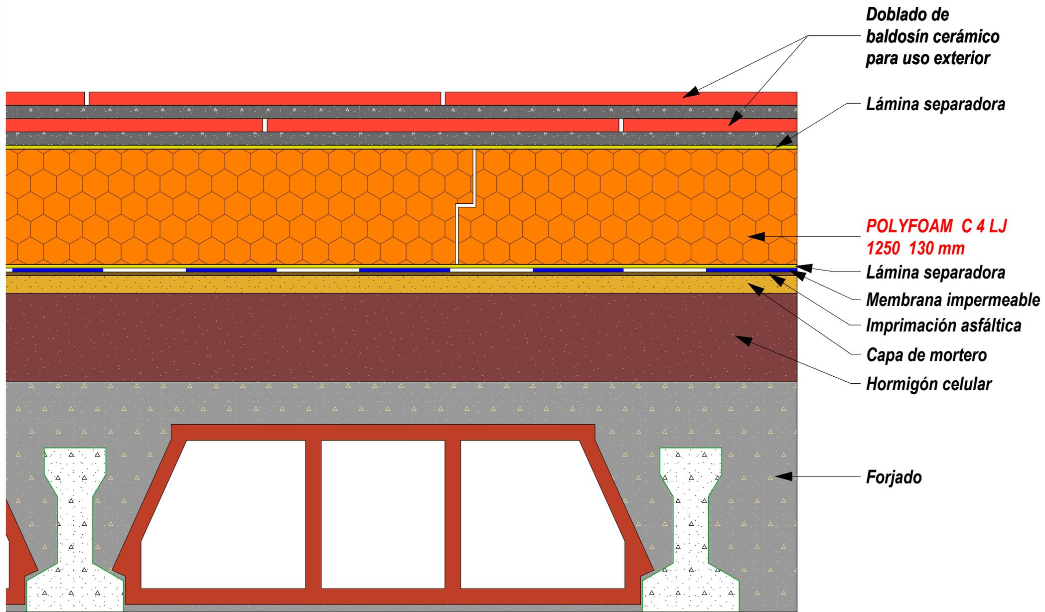
**CUBIERTA INVERTIDA CON SOLADO Y POLYFOAM C4 LJ 1250 (Transitable)**
